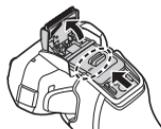
Press and hold the lock release button (a) and slide the trimmer handle down to lower the trimmer.
