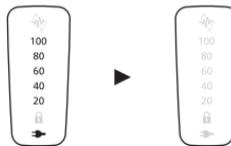
The battery capacity lamp and the charge status lamp (➔) will light up and then turn off after 5 seconds.
