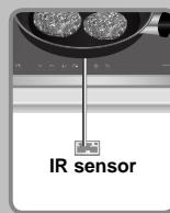
The **IR sensor of Panasonic** (Temperature control system) regulates set temperatures by quickly detecting the temperatures on the bottom of the cookware, so it is easy to prepare delicious food.
