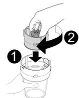
Make sure the mill gasket is not damaged and placed properly before assemble.
