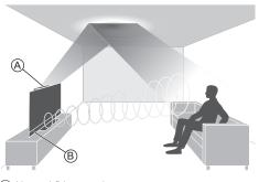
(A): Upward-firing speakers (B): Left-center-right speakers
