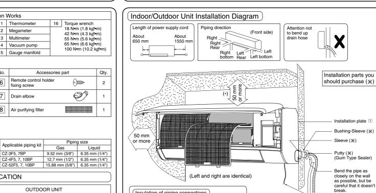
(Insulation of piping connections ) Carry out insulation after checking for gas leaks and Vinyl tape (wide) (※) X Vinyl tape Apply after carrying Attaching the remote control holder to the wall Remote control holder fixing screws 6 Remote control holder 5 - Saddle (※)
