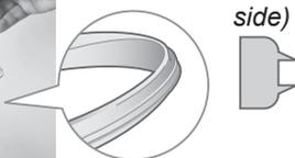
Ensure that the rubber seal is not inside out when re-fitting. If the seal is not fitted correctly the lid will not close securely and it will leak.
