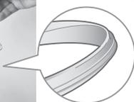
Ensure that the rubber seal is not inside out when re-fitting. If the seal is not fitted correctly the lid will not close securely and it will leak.
