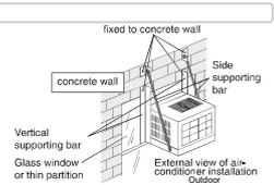
This can minimize the noise problem caused by improper installation.
