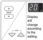
Press TEMP ▲ or ▼ to set the display temperature. The temperature can be set between 16°C and 30°C. Recommended temperature: 26°C-28°C
