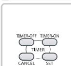
When the air conditioner is OFF: Press the TIMER-OFF button to set the timer. Press the same button until the preferred hour of operation is reached. (The TIMER indicator light will blink to await for setting) Press TIMER SET button to complete the setting. At this time, the TIMER indicator light is steady instead of blinking.
