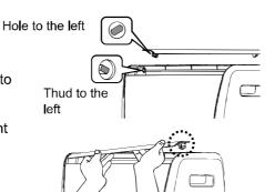
Turn the louver upward and downward for easy inserting
