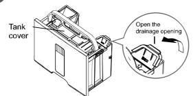
Carry the center part of water tank handle and hold the bottom part to drainage position.
