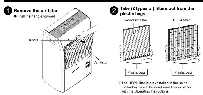
3 Installation procedures: attach the deodorant filter first, and then attach the HEPA filter.
