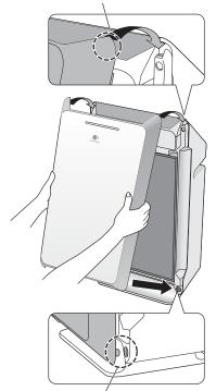
Push in the protrusion into the holes (2 places) of product and press properly.
