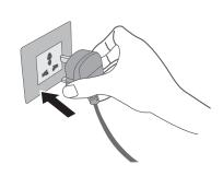
■ When inserting the power plug, as the odor sensor uses the degree of cleanliness at this time as the standard, we recommend that you plug it in when the air is fresh (when there is no cigarette smoke). (The standard of the odor sensor automatically updates itself according to the degree of the indoor cleanliness.)
