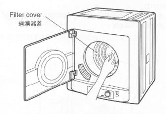
Detach the back-filter B and the filter from the filter cover.
