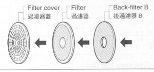
Fit the concave portion of the center of the filter cover onto the convex portion of the center of the drum and fasten securely.
