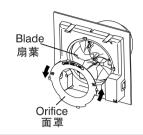
Wash and clean the louver, the orifice 清洗百葉窗、面罩。
