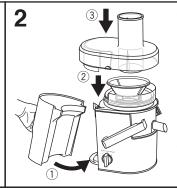
Attach the Pulp Container and make sure it is fully aligned with the body.
