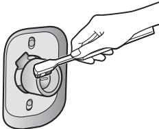
7. Disconnect the hose from the tap and then clean the filter on hose in the same way.
