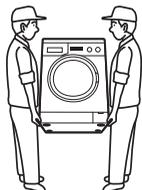
Start by tilting the appliance backwards. The appliance should be carried by two people, one on each side holding it from the bottom.
