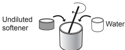
Rinse out the remaining softener with a splash of water or a damp cloth after washing. If it sticks to the compartment, pull out the drawer and clean it out. (PP.28-29.)
