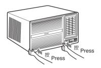
Put back the air filter and cover with the front intake grille.
