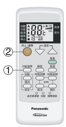
DRY mode is to give a gentle cooling operation at low fan speed to reduce the humidity in the room.
