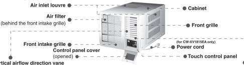
Vertical airflow direction vane (Airflow direction adjustment up-
