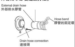
Connect the drain hose securely to the main body of the washer.
