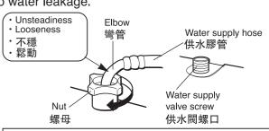
Firmly tighten the nut. Otherwise, it will result in water leakage.
