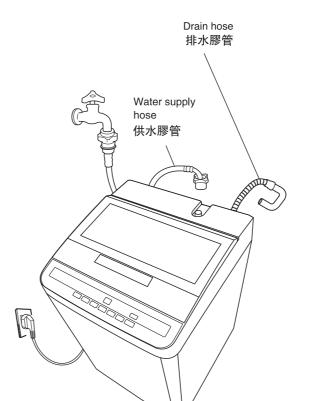
Connect the water supply hose to the water supply valve screw.
