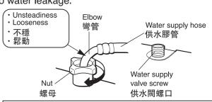
Firmly tighten the nut. Otherwise, it will result in water leakage.
