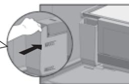
Hold the water supply tank horizontally. Confirm the direction of the water supply tank and install it firmly. (If the water supply tank is tilted, water may spill out)
