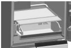
Pull out the case quickly, raise the front end, and then hold the upper edge of the case and pull it out obliquely.
