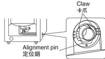
4 Install the hose hole cover to the right hose hole, and fasten with the screw.
