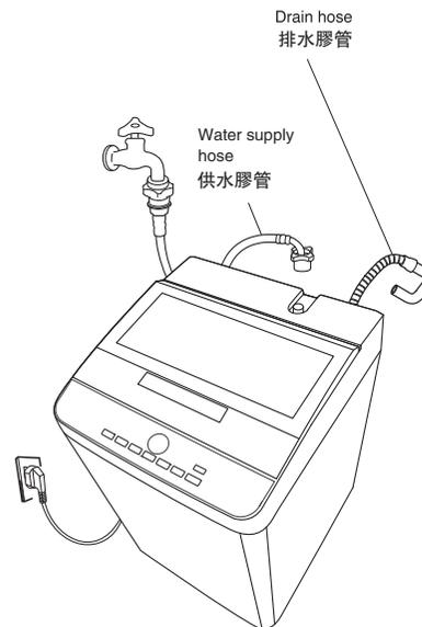
Connect the water supply hose to the water supply valve screw.
