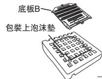
**1** Remove the bottom plate adhered on the side cushion of the washing machine.
