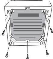
**3** Align the bottom plate with the tabs of the outer edge of the frame(3 tabs) and install by fastening screws at 5 locations. (Only for NA-F80G9P)
