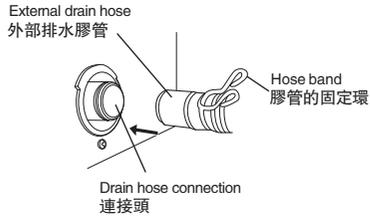
1 Connect the drain hose securely to the main body of the washer.
