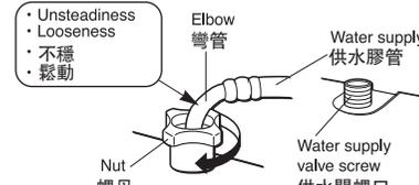
Firmly tighten the nut. Otherwise, it will result in water leakage.
