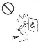
Unplug roughly may damage the power cord, cause electric shock. short circuit fire.
