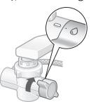
② Loosen the nut, remove the bypass selector, and take out the gasket and filter.
