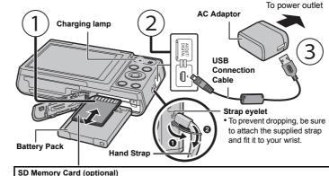
The following cards, which conform to the SD standard, can be used with this unit.
