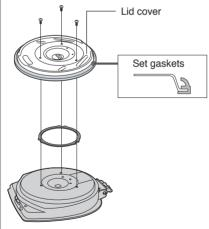
Remove lid, unscrew 3 tapping screws and remove the lid cover. Exchange the gaskets and then place the lid
