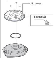
Remove lid, unscrew 3 tapping screws and remove the lid cover.
