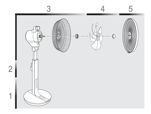
安裝後保護網 安裝架子 裝上遙控器支架 安裝扇葉 安裝前保護網 ▶8頁 ▶9頁 ▶9頁 ▶8頁 ▶9頁 Installing the stand Attach the remote Installing the rear guard Installing the blade Installing the front guard ► P.8 control holder ▶ P.9 ▶ P.9 ▶ P.8 ▶ P.9
