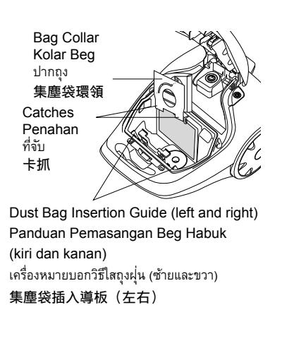
② Push the Bag Collar in the direction of the arrows shown in figure until it catches on the Hooks and close the Dust Cover.
