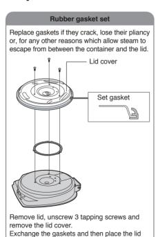
cover back and secure with the tapping screws.
