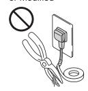
Damage from heavy objects placed on top, heating, or pulling could cause fire or electric shock.
