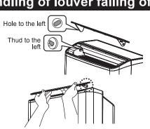
Turn the louver upward and downward for easy inserting
