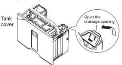
Hold water tank handle and its bottom to drain it.
