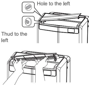
Turn the louver upward and downward for easy inserting
