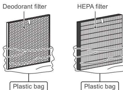
※ The HEPA filter is pre-installed in the unit at the factory, while the deodorant filter is placed with the Operating Instructions.
