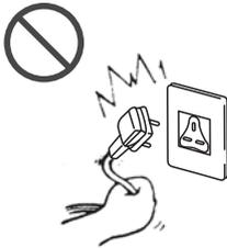
Unplug roughly may damage the power cord, cause electric shock, short circuit fire.
