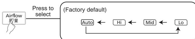
※ The airflow can adjust when in Fan mode. Only Airflow in Auto mode, the air flow will be changed by the volume of PM2.5 and maloder.
