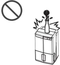
Water may spill into the unit and fire or electric shock may occur.
