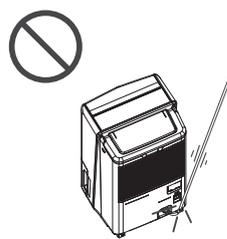
It may cause short circuit or broken wires (which may cause fire or electric shock.)
