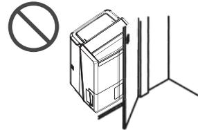
If there is insufficient ventilation, overheating and fire may occur.
