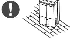
If the unit tilts, water will overflow, and wet the property potentially causing fire or electric shock.
