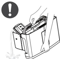
Leaked water may damage the household items and property damage even cause accident. (People may be injured and caused fire or electric shock.)
