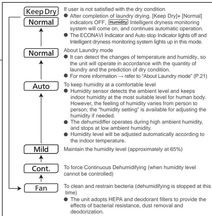
\* When the filter is detected by the filter detector, the [Fan] will light up as you press down the Function selection. If no filter is installed, the [Fan] will not light up when the Function selection button is pressed. The [Fan] will light up when only the air purifying function is in operation. The air velocity may vary depending on the use of the HEPA filter.
