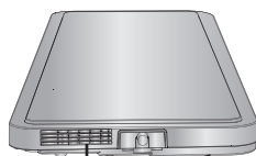
Intake port (Right side, bottom)
