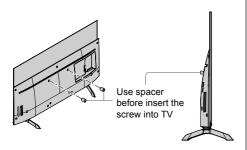
Holes for wall-hanging bracket installation Rear of the TV
