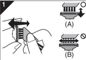
1. Clean the inner blades using the short brush by moving it in direction (A). Clean the outer foil, the shaver body and the trimmer using the long brush.
