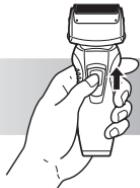
**1** Depress the switch lock button and slide the 0/1 switch upwards.
