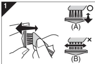
1. Clean the inner blade using the short brush by moving it in direction (A). Clean the outer foil, the shaver body and the trimmer using the long brush.
