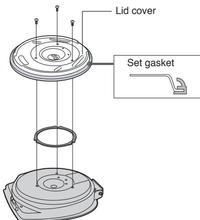
Remove lid, unscrew 3 tapping screws and remove the lid cover.
