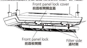
Composite and deodorizing filter (front side (active carbon side) faces upward) 集塵脫臭過濾網(正面(活性碳側)朝上)
