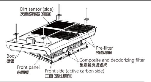
Composite and deodorizing filter (When the filter clean indicator is on (about once a month))
