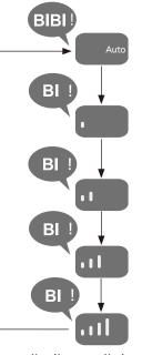
Auto (automatically adjust the air volume according to the air pollution detected by sensor, and use appropriate air volume to purify air.)
