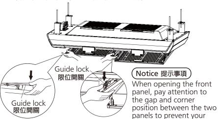
fingers being clamped. 打開前面板時,請注意 兩面板間的間隙及邊角
