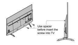
Holes for wall-hanging bracket installation
