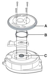
Remove lid, unscrew 4 tapping screws and remove the lid cover. Exchange the gaskets and then place the lid cover back and secure with the tapping screws.
