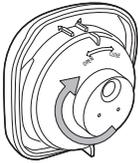
Fold and press it firmly. When a clear sound is heard, it indicates completion of assembly.
